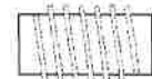
Wood Thread to Machine Thread Bushing For J or M Mountings on Wood Doors B3 - 1/4-20 Thread B4 - 5/16-18 Thread B5 - 3/8-16 Thread
